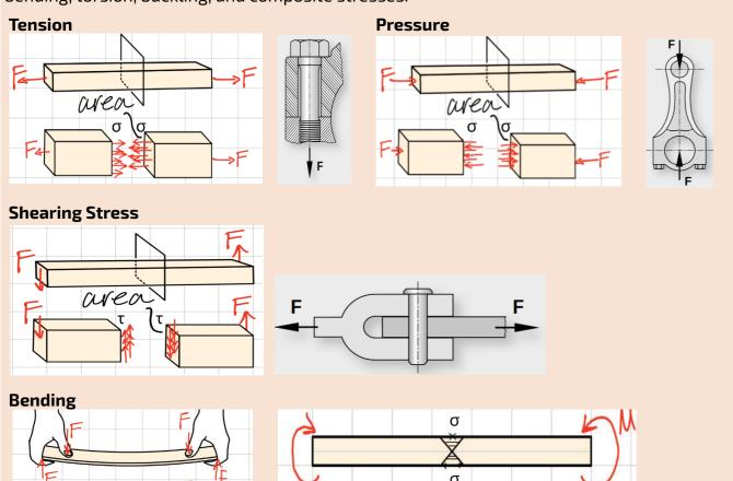
**F** - force, **M** - moment, **M**t - twisting moment,  $\sigma$  - stress,  $\tau$  - shear stress
