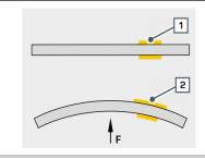
F force, 1 strain gauge in component not under load, 2 strain gauge in
